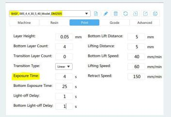
Figure 5: Material specific setting of various parameters such as exposure time in the Chitu Box V1.8.1 Slicing Software. (Source: Organical CAD/CAM)
