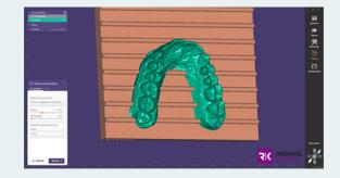
Figure 6: Creating the hollow model with exocad® Model Creator.
